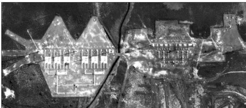
**Figure 2:** The two transmitter antennae of the HF 1 MW OTH *PLUTO* System at Akrotiri in the Western Sovereign Base Area (WSBA) – installed in 1998 (*PLUTO* I antenna, height 58 m) and 2002-2003 (*PLUTO* II antenna, width 196 m and height 96 m) – provide the capability of monitoring strategic activities in the Asian heartland at a range of 5000+ km. © 2015 Google Earth.
